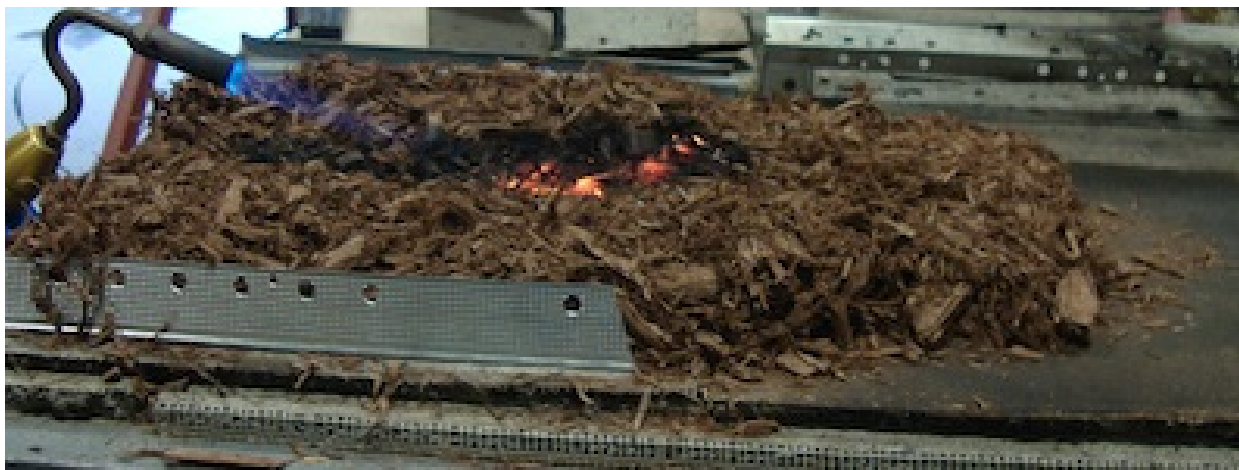
6:40: Slight glowing; no flame or smoke: concavity 3/4"
