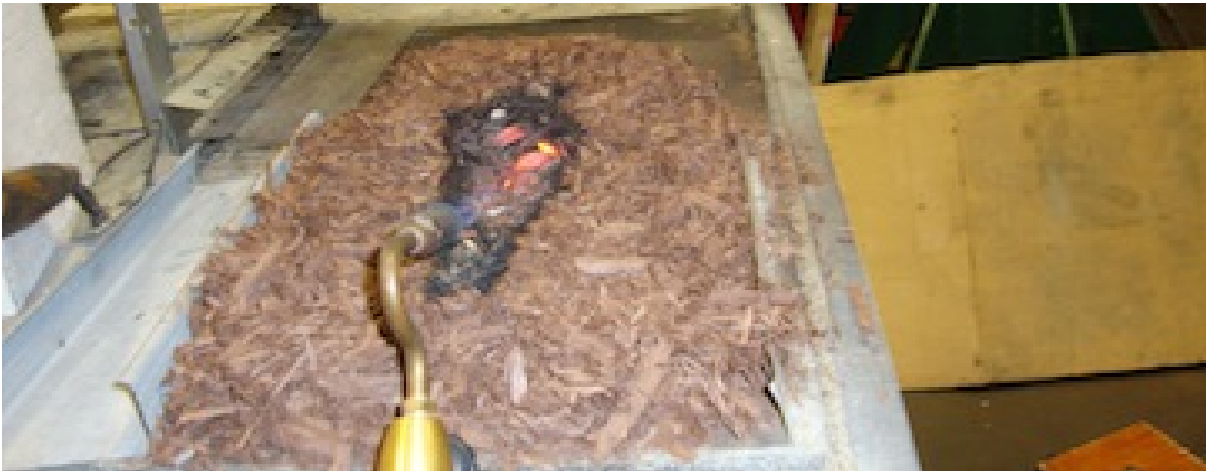
9:00: View from torch end showing glow in concavity of 1"
