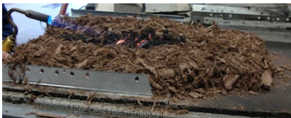
1:19: No flame spread beyond torch area concaving
